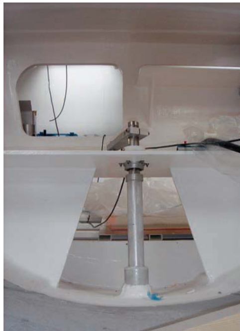
above Well braced on top and at the bearing end, this aluminum rudder post will provide years of service and even resist minor impacts with floating objects.
