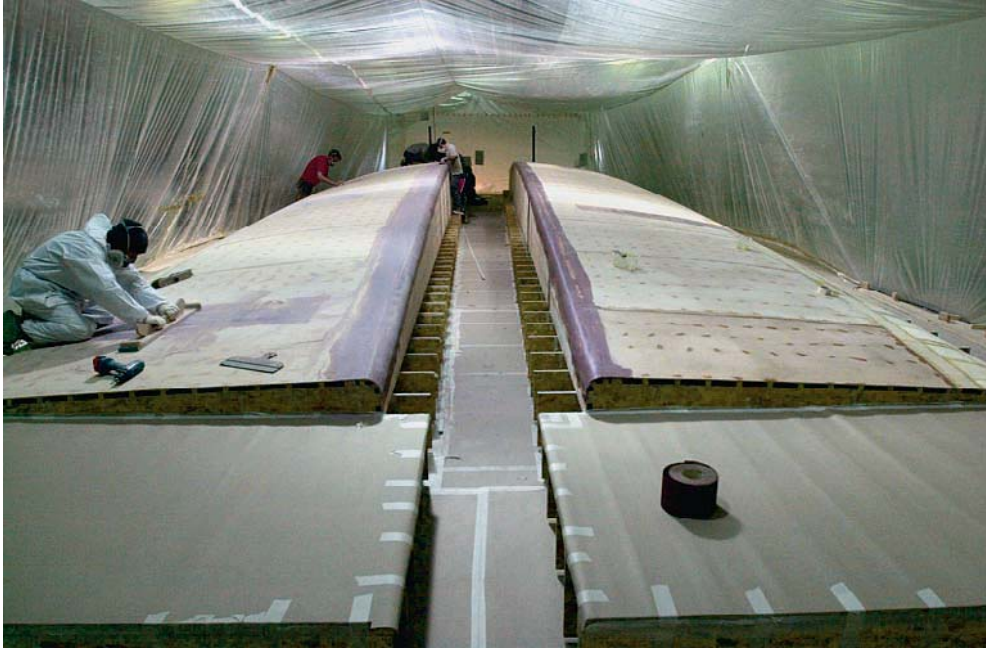
above Split hull plugs of a Blubay 72 are filled and faired; a time-consuming and tedious process, but necessary for exacting results.
