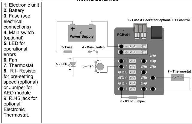
NOTE: When using the modular thermostat connection (#9) there are no connections on thermostat terminals (#7).
