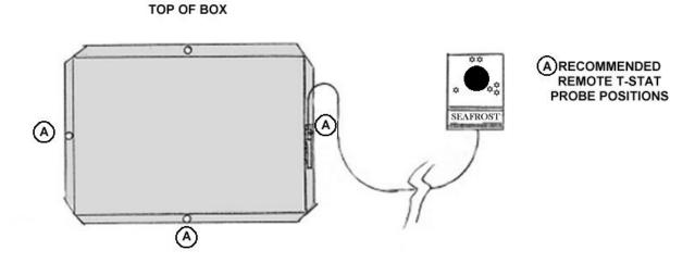
For the best operation pull excess thermostat sensing tube into the insulated space. This can be coiled.
