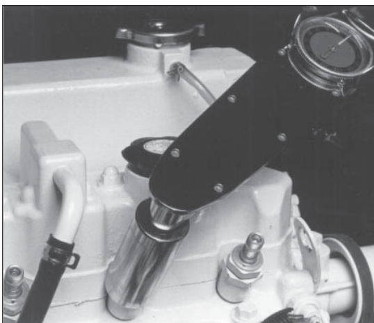
Figure 18: Reinstall injector. Torque to proper tightness.
